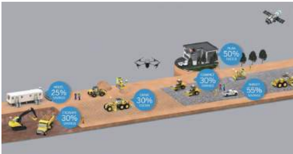
Figure 2: Trimble-published efficiency gains across the earthworks cycle, underpinned by GNSS satellite positioning (source: Trimble Earthworks Solutions).
